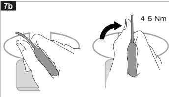
With Torque Key inserted, turn clockwise until handle straightens out as shown above. This indicates 4-5 Nm. More pressure may be required in extreme climates.
